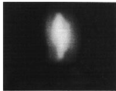
Figure 2. Blue light emission emanating from bulk nanocrystalline GaN powder (sample a) upon 325 nm excitation.
